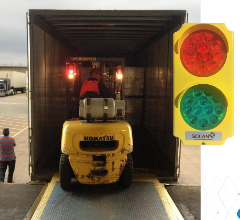
If the driver will decide to move the i-Stop there will be immediate two kinds of alerts: a 5/10/15 second alarm horn warning that will allow the forklift driver to get out of the truck and back to the platform safely. In addition, a red LED light will appear indicating that whoever is currently inside the truck must return to the platform.
