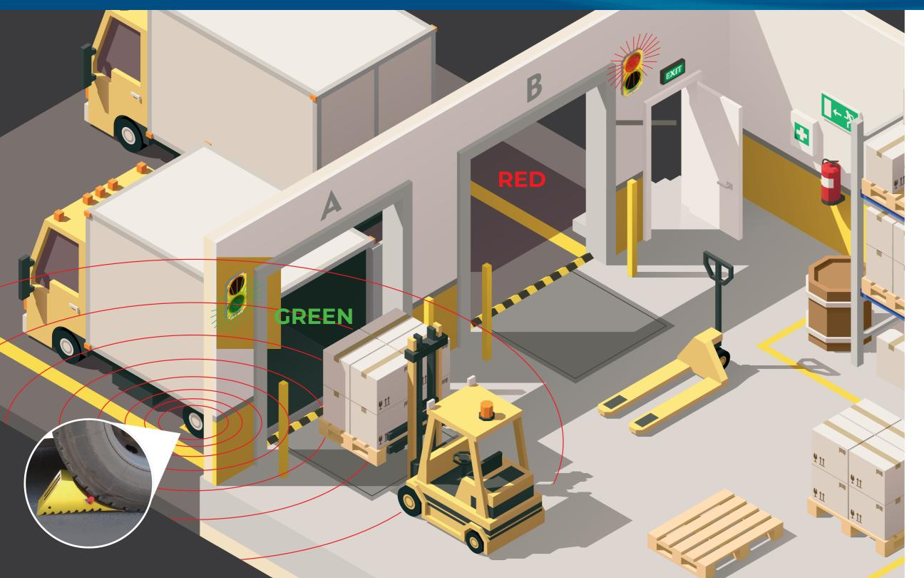
With Solan i-Stop System a truck will no longer move with a forklift inside.
